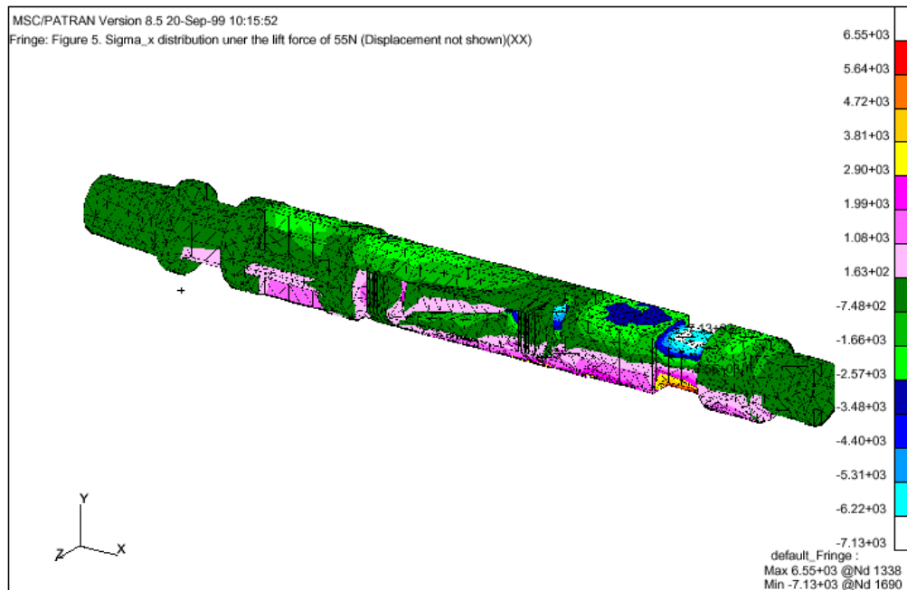
Figure A. 5: x component stress distribution in psi when a lift force of 12.36\ lb is applied at the tip.
