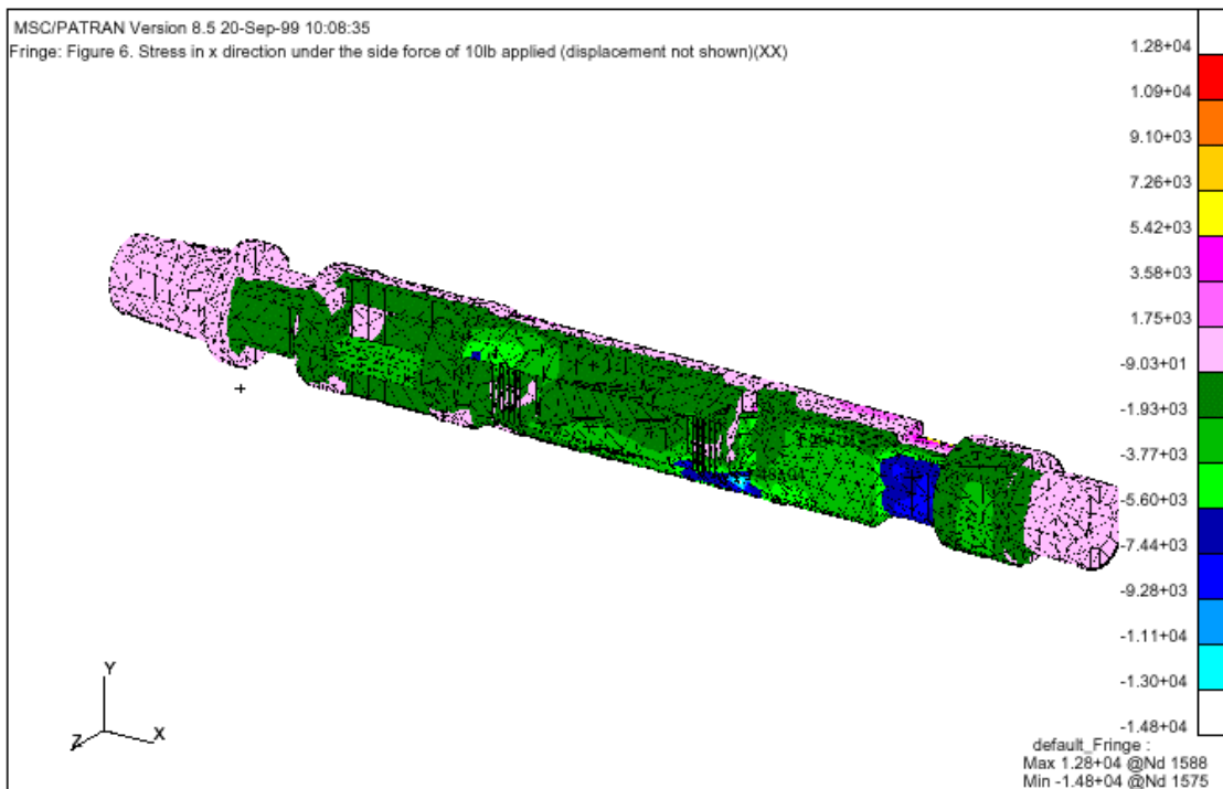
Figure A. 8: x component stress contour in psi when side force of 10\text{ lb} is applied at the tip.
