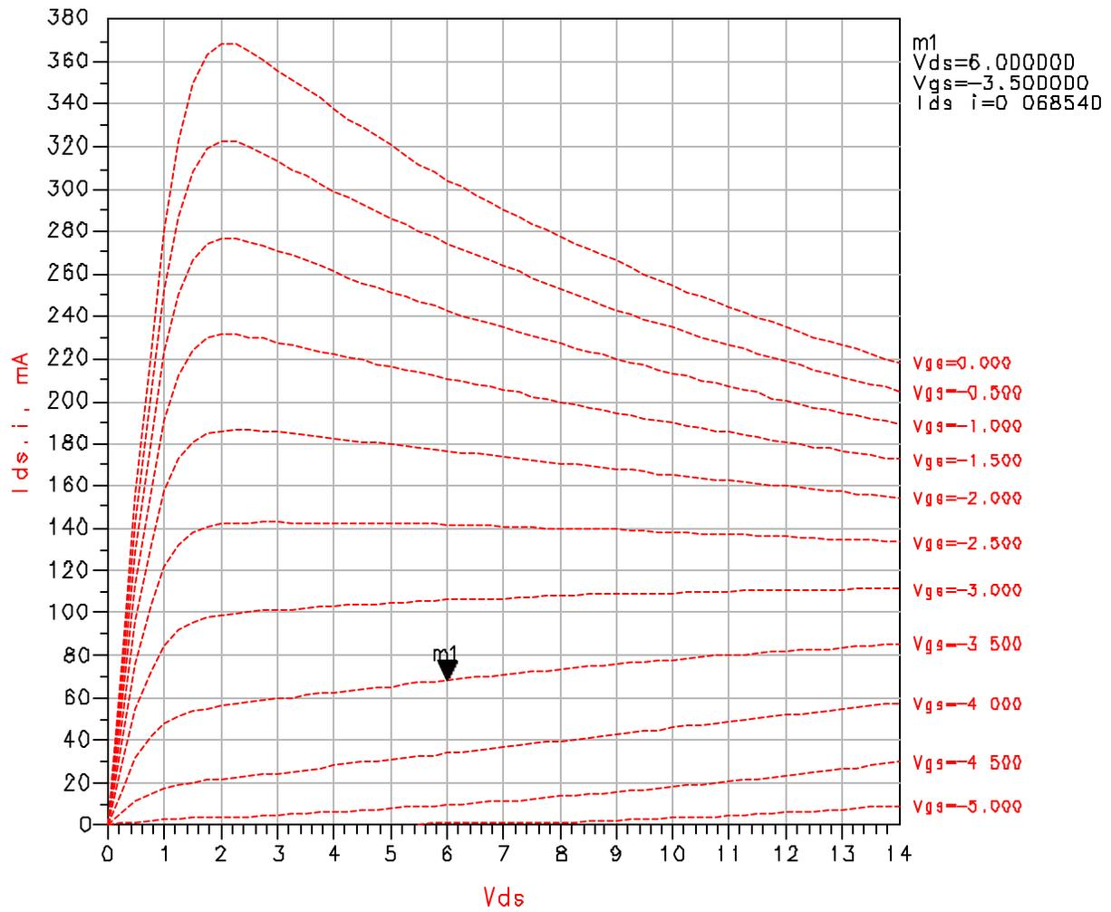
**Figure 4.2** DC curve tracer for the ATF-46100
