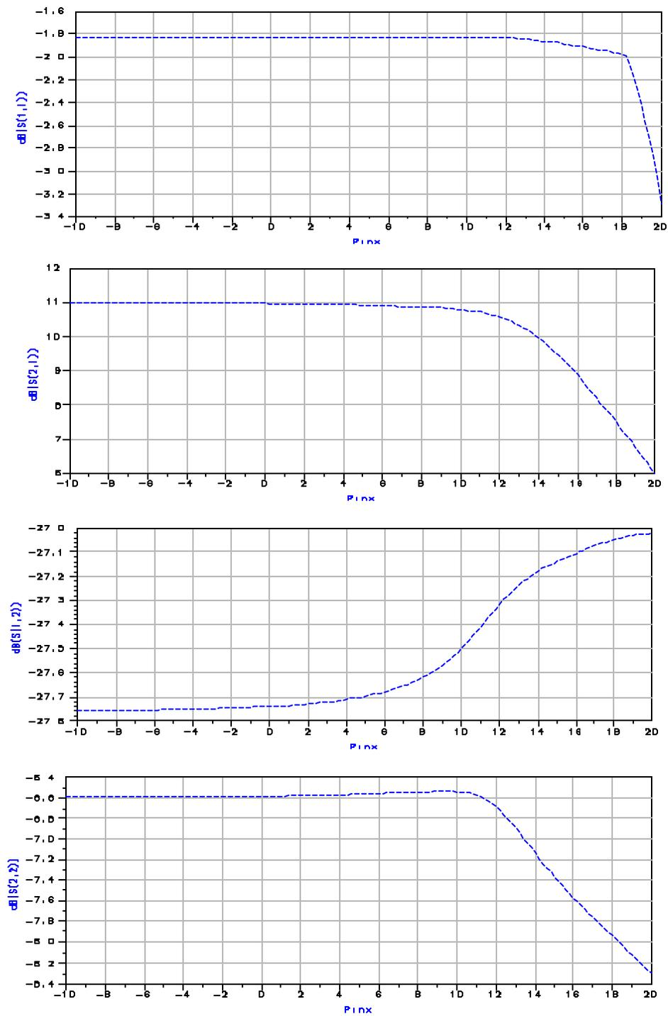
Figure 4.4 (a) S-parameters in dB vs. the input power.
