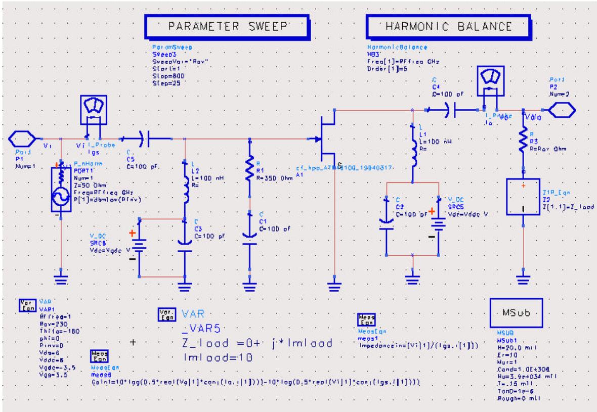
**Figure 4.5** Harmonic balance simulation setup for the gain.
