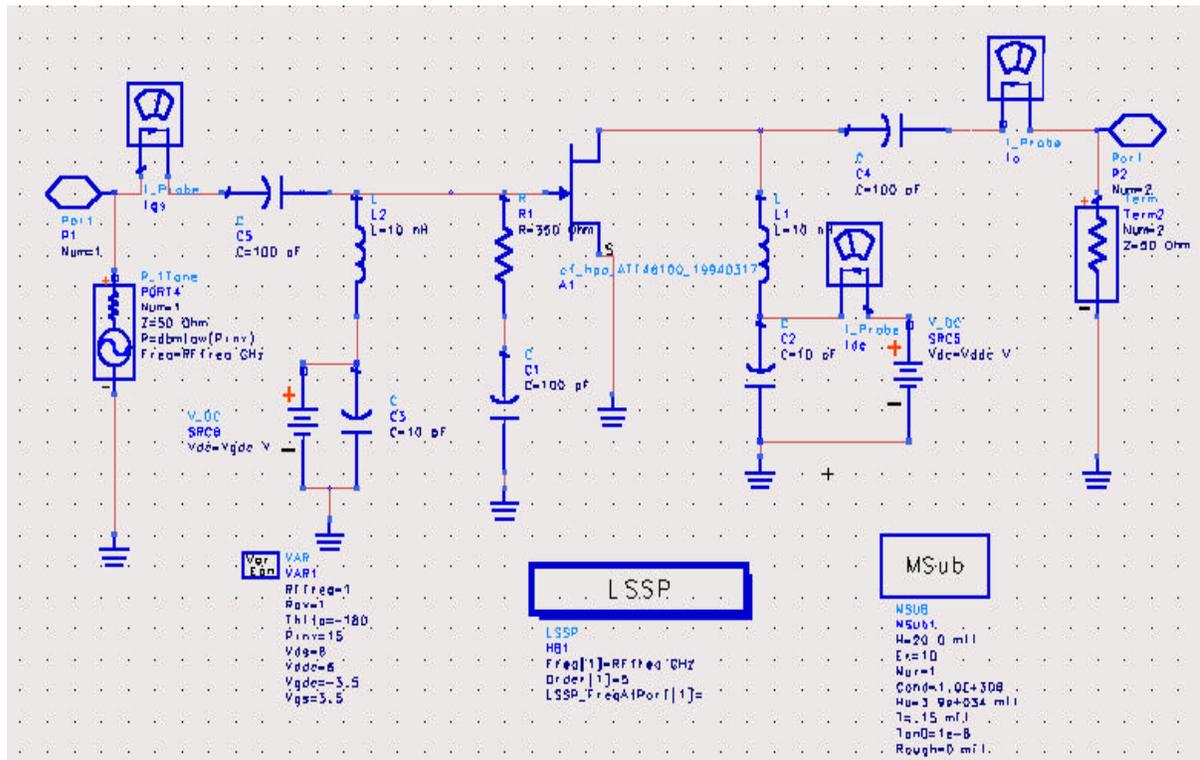
Figure 4.3 S-parameters simulation setup for the ATF-46100.
