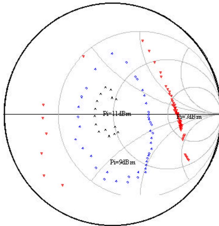
**Figure 4.7** 0.2 dB Compression point vs. input power.
