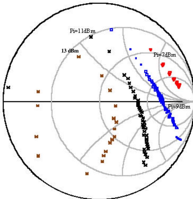
**Figure 4.6** 1dB Compression point Vs input power.
