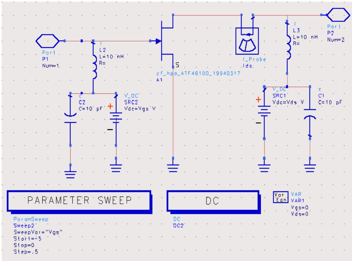
**Figure 4.1** ATF-46100 DC simulation setup.
