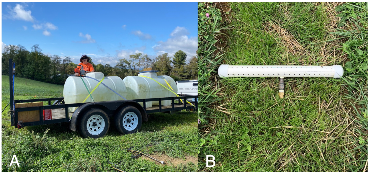
Figure 3.6. (A) Simulated flow set up shows two tanks, containing the nutrient amended solution, on trailer and an Echo pump. (B) Flow spreader within ditch that was attached to hose from Echo Pump during simulated runoff events.
