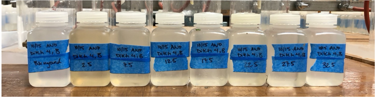
Figure 4.7. BT samples prior to filtering. Clear color differences can be seen between samples taken at the beginning versus the end of the experimental run.
