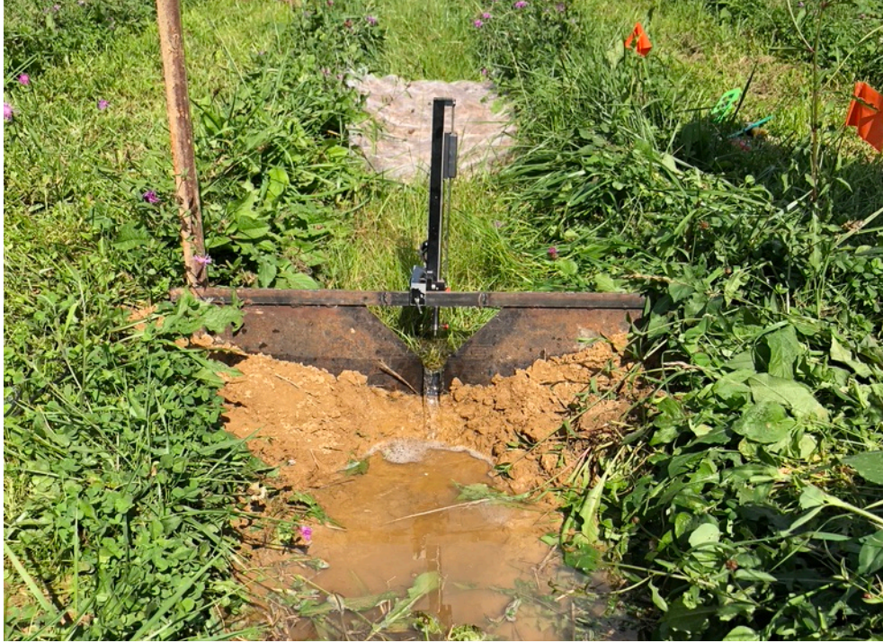
Figure 3.7. Outlet flow measuring device, including weir and point gauge, during simulated runoff event. Bioreactor is visible behind the point gauge.
