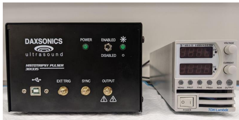
Figure 2.9: Custom histotripsy pulser (left) power supply & amplifier (right) by Daxsonics for coaxial setup. The FUS transducer connects to OUTPUT, the function generator connects to EXT TRIG, and the power supply mediates the output to the transducer.
