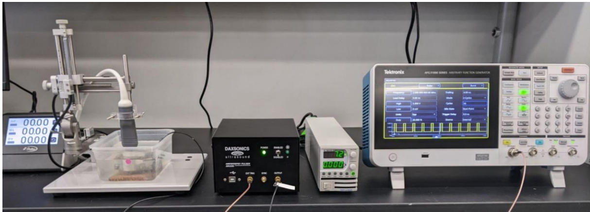
Figure 2.11: Coaxial experimental setup (left to right): stereotaxic position electronic readout, stereotaxic stage with FUS and imaging transducers, mouse in degassed DI water bath, Daxsonics histotripsy pulser, power supply / voltage regulator, function generator.
