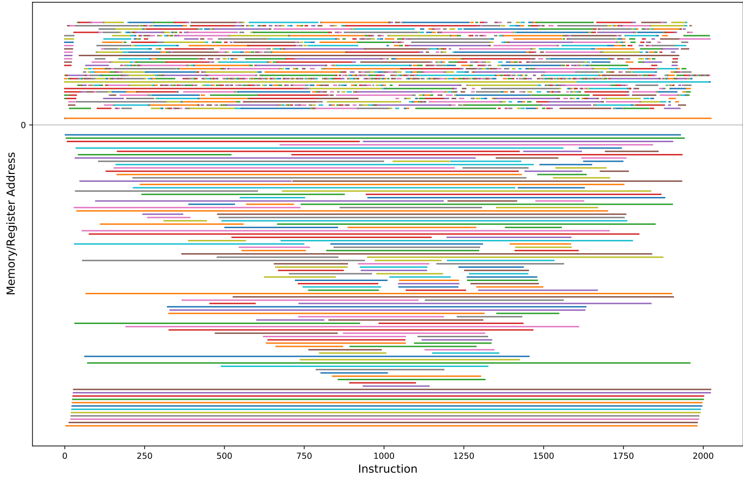
Figure 5.4: Register/Memory usage of the 8-bit MAC PSP function [used with permission] © 2020 IEEE
