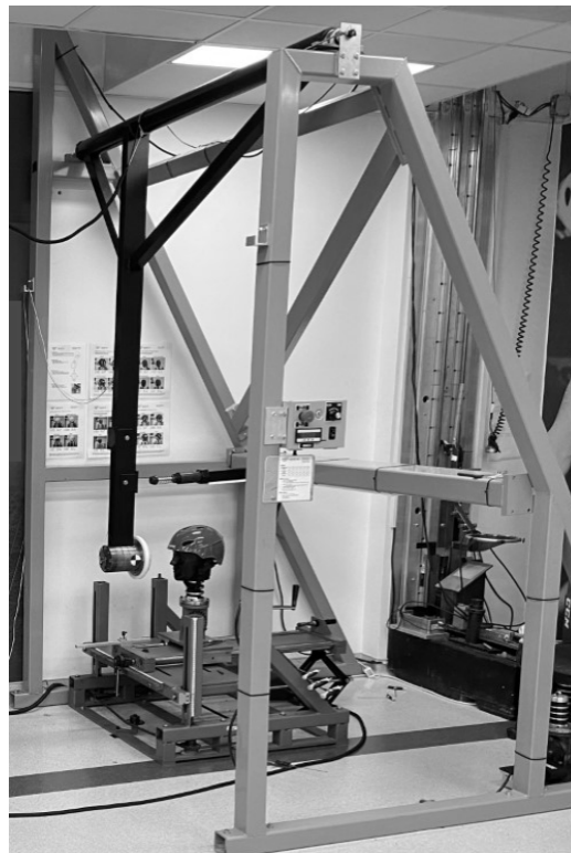
Figure 1: Pendulum impactor used for Whitewater STAR testing.
