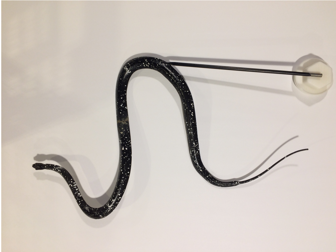
Figure 2.1: This is a photo of the 3D printed snake model showing the painted black background and the speckle painted calibration pattern. A stainless steel support cantilever beam holds the model in place during experiments.
