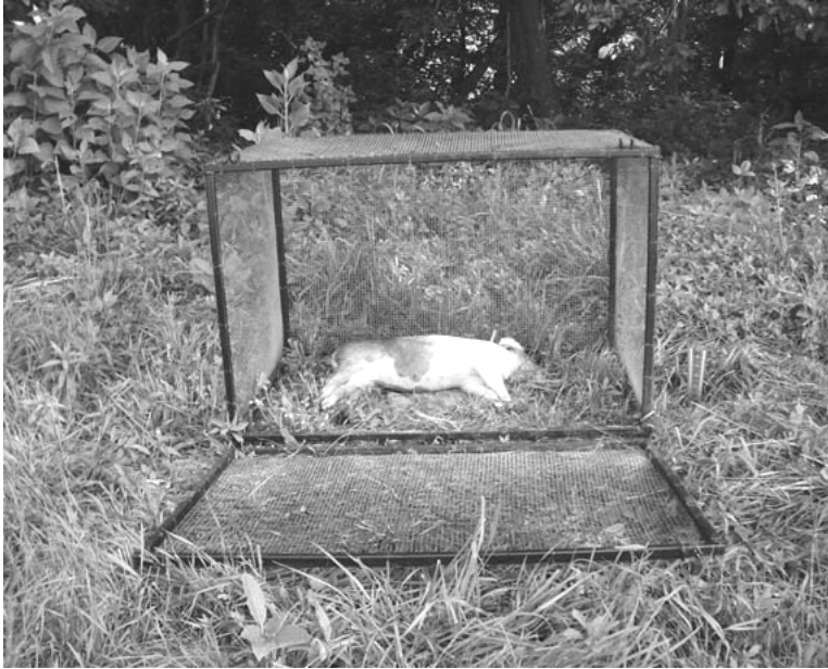
Figure 4.1: Cage (with an open-bottom) used to isolate pig carcasses during succession studies. Hinged door at the front of the cage provided easy access to the carcass during the study
