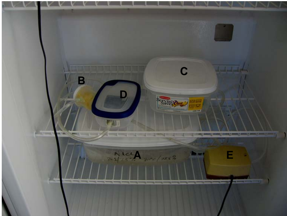
Figure 6.1: Relative humidity chamber used for collecting egg hatch data for Phormia regina and Phaenicia coeruleiviridis (A: salt chamber, B: filter chamber; C: egg chamber; D: data logger chamber; E: pump)
