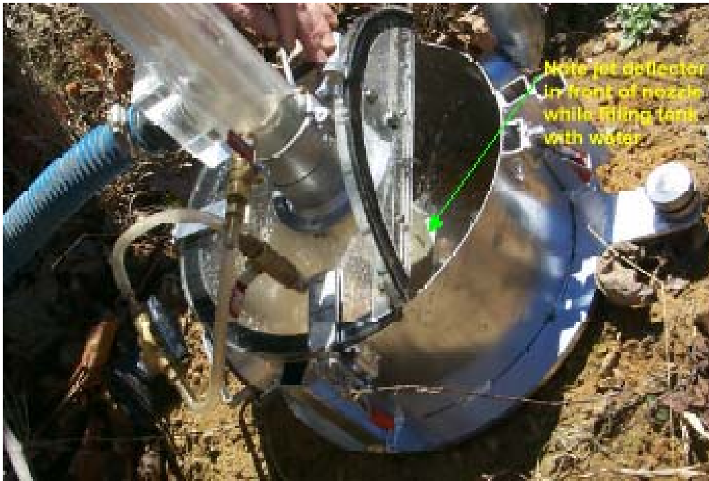
Figure G4. Filling tank with water prior to start of jet test (picture courtesy of Dr. Greg Hanson, Research Hydraulic Engineer, USDA-ARS Hydraulics Engineering Research Unit, Stillwater, OK).
