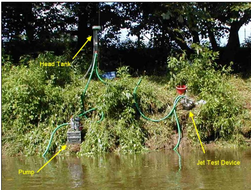
Figure G3. Jet test setup at site EL1.
