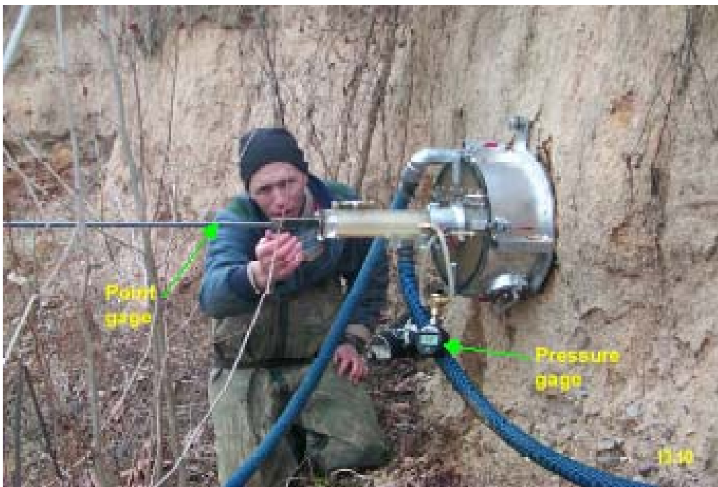
Figure G5. Taking point gage reading on bank. (picture courtesy of Dr. Greg Hanson, Research Hydraulic Engineer, USDA-ARS Hydraulics Engineering Research Unit, Stillwater, OK).
