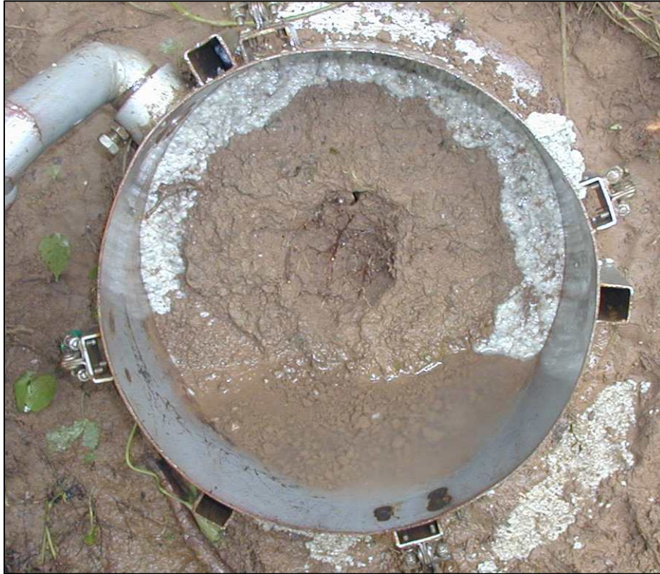
Figure 5.8. Eroded aggregates at bottom of jet test tank.
