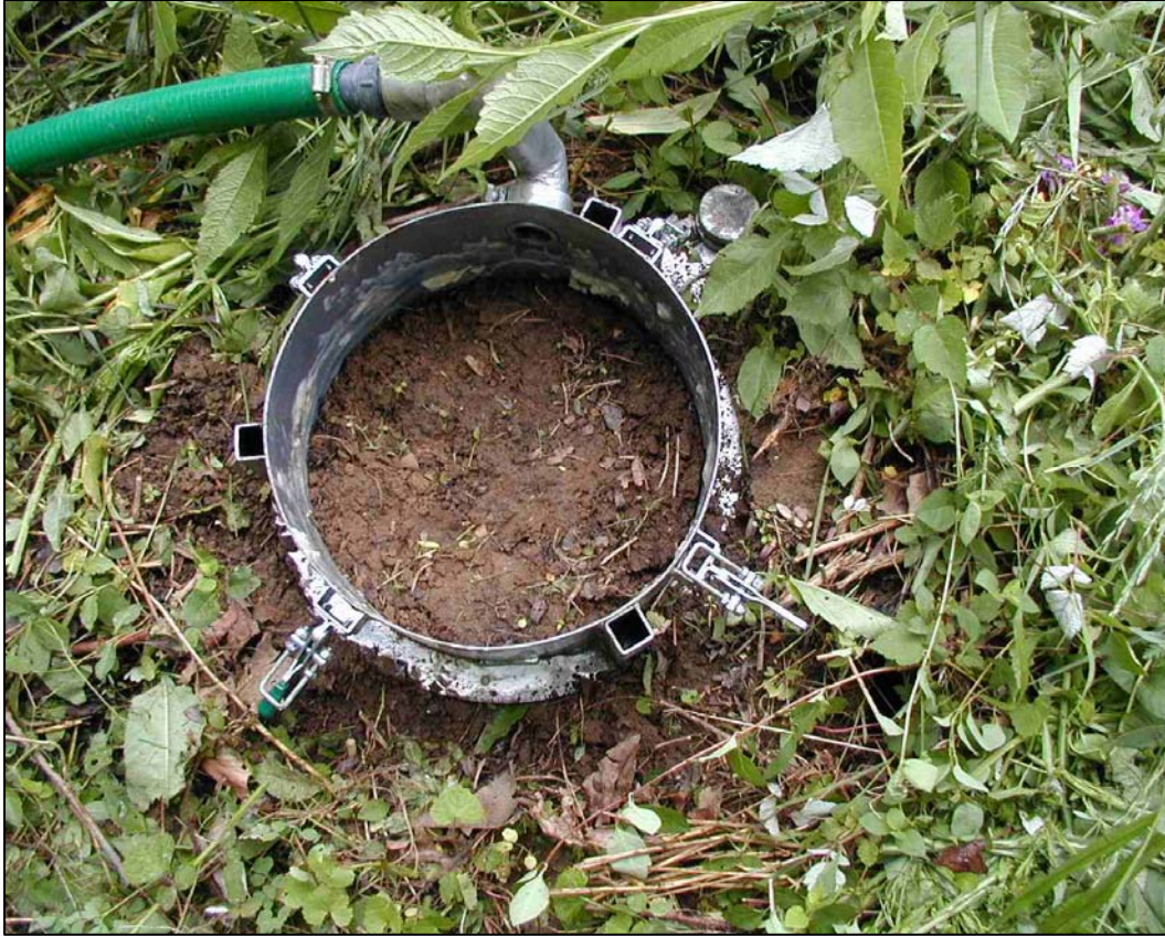
Figure 5.3. Prepared bank surface prior to jet testing.
