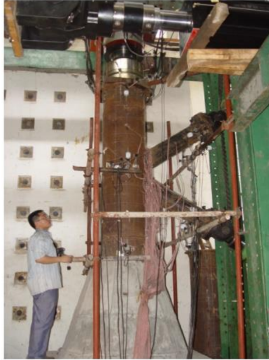
Figure 2.15 View of a K-connection sample and of the test set-up from Huang et al. (Huang et al., 2015)
