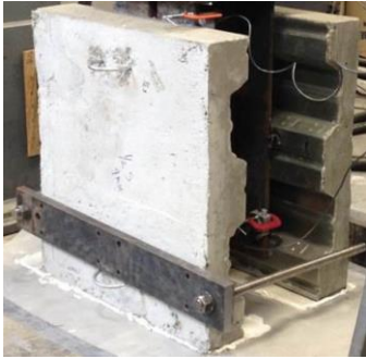
(b) Experimental model for a push-out test.
