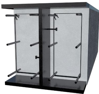
Figure 1.3 Some possible configurations of steel and concrete composite members.
