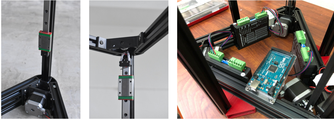
(a) Stepper Motor (bottom) and Linear Carriage (top)
