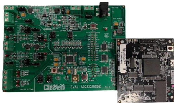
Figure 4.17: Resolver development and evaluation setup
