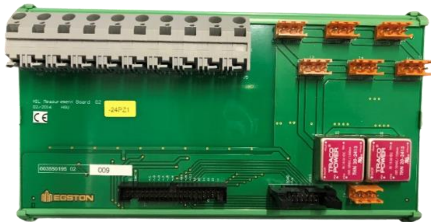
Figure 4.11: Modified EGSTON signal conditioning board (for OPAL-RT)
