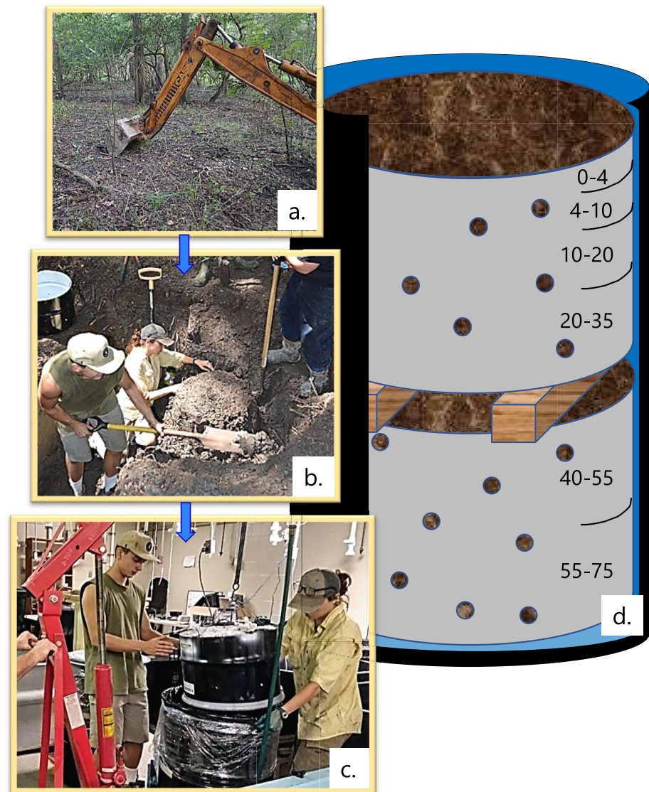
Figure 1. Sampling and experimental setup: (a) initial excavation of a trench; (b) manual excavation of a monolith adjacent to the trench; (c) lowering a monolith into a tank of artificial floodwater; (d) schematic of the paired monoliths in perforated containers submerged in artificial floodwater, omitting the thin, open-weave, cotton cloth wrappers around each ped.
