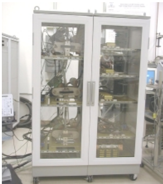
Figure 4-20 One megawatt three phase voltage source inverter system using ETO1045S.
