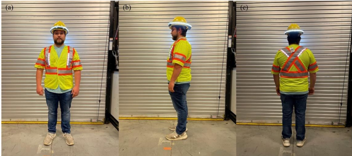
Figure 5. Photo. Simulated worker in the Class 3 vest with white LEDs and helmet-mounted LEDs.
