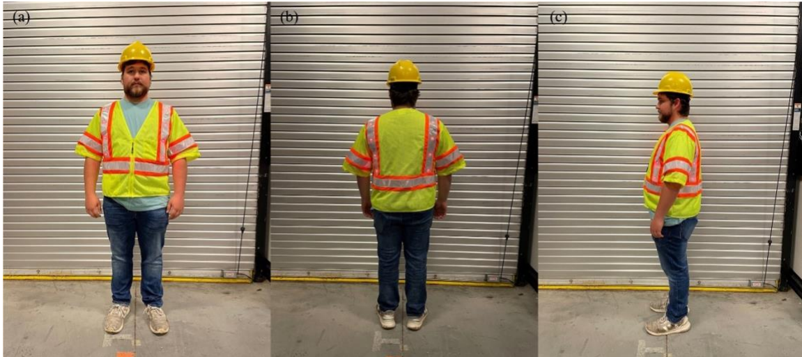
Figure 3. Photo. Simulated worker in the Class 3 vest with red LEDs.
