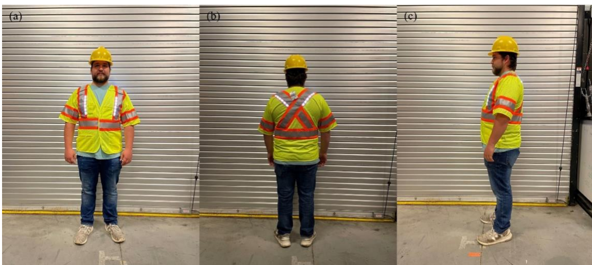
Figure 2. Photo. Simulated worker in the Class 3 vest with white LEDs.
