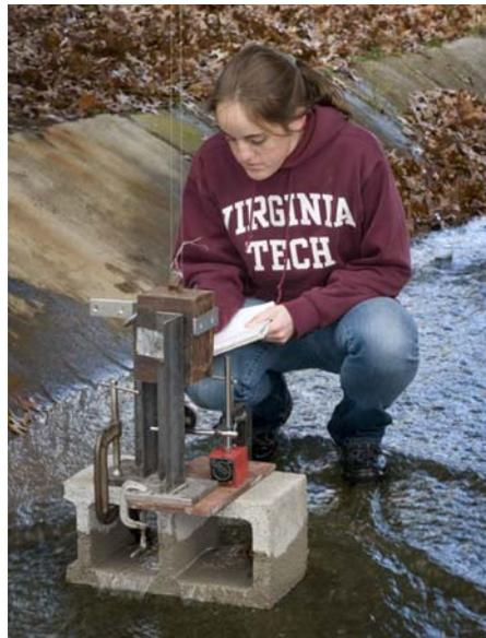
Figure 13 Test set up with dial gage, weight, and steel guides
