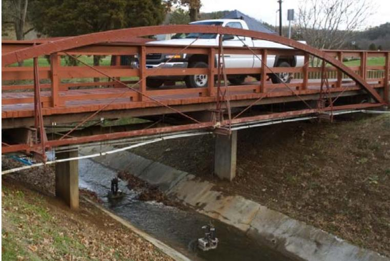
Figure 14 Load test in progress. The truck is centered transversely across the width of the bridge and two dial gages with stands are below the midpoint of each truss.
