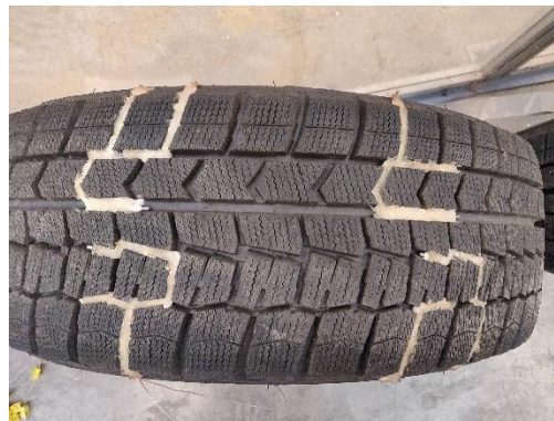
Figure 8: Tire after fixing of thermocouples in the grooves
