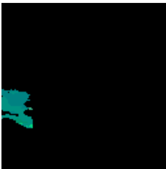
Figure 3.16: An outlier grain from the experimental z_{xz} data of Figure 3.15. Here, the orientations of all pixels are very similar. As a result, the clustering algorithm considered them to be the same grain. [60]
