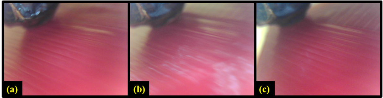
Figure 5.8: (a) Surface quality in Geometry 1 with optimal parameter setting for Geometry 1 (target surface quality); (b) Surface quality in Geometry 2 with optimal parameter setting for Geometry 1; (c) Surface quality Geometry 2 with optimal parameter setting for Geometry 2.
