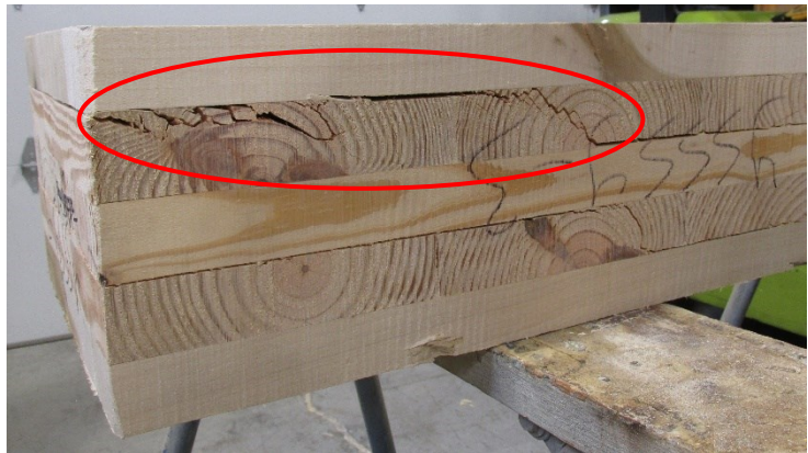
Figure 15. Example of rolling shear failure of tested CLT beams
