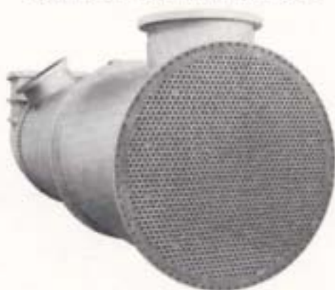
AIR-TO-AIR HEAT EXCHANGER WITH 2000 STEEL TUBES EXPANDED AND SEAL WELDED TO TUBE SHEET.
