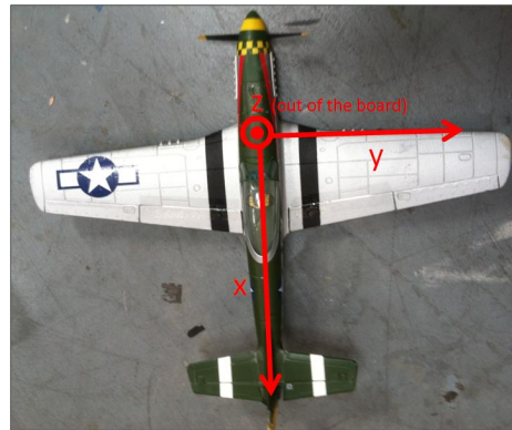
Figure 6.15: AVL coordinate system for a typical aircraft
