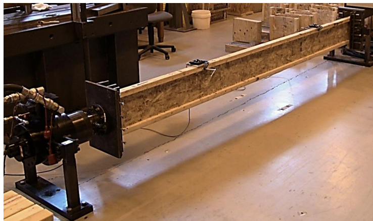
Figure 4-7: Torsional rigidity test configuration (inches).
