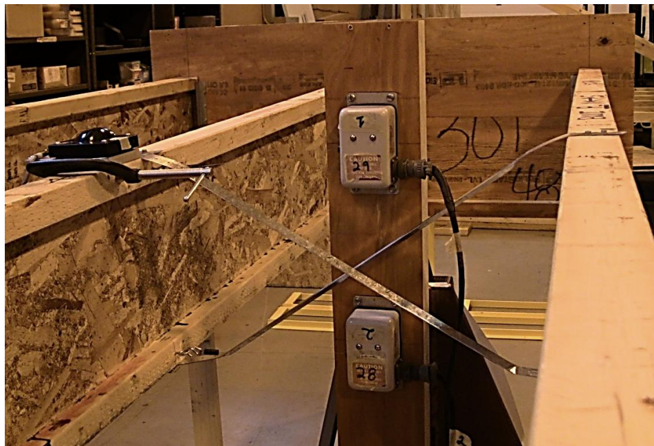
Figure 4-8: Static lateral-torsional buckling test configuration (inches), a) isometric view, b) front view.
