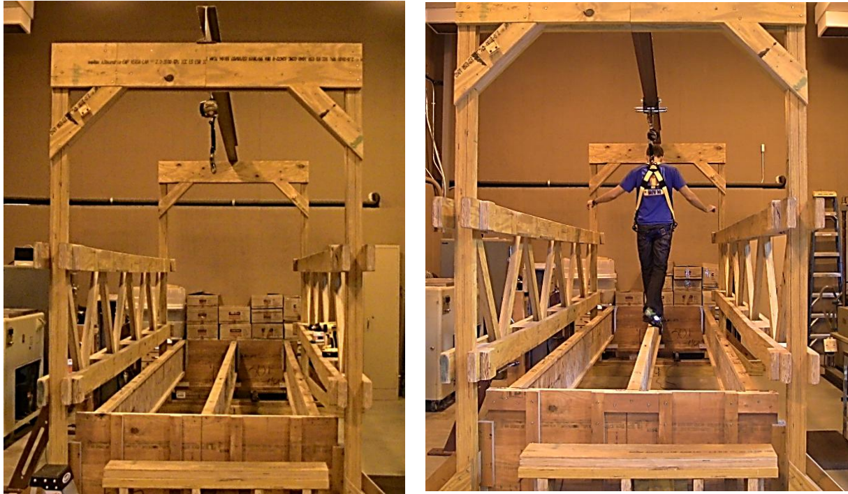
Figure 5-14: Photographs showing the walking platform (left) and a participant walking on a wood I-joists (right).
