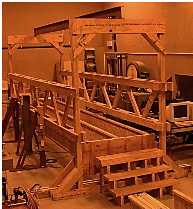
Figure 4-9: Safety platform used in the dynamic lateral-torsional buckling tests (approximate dimensions in inches).
