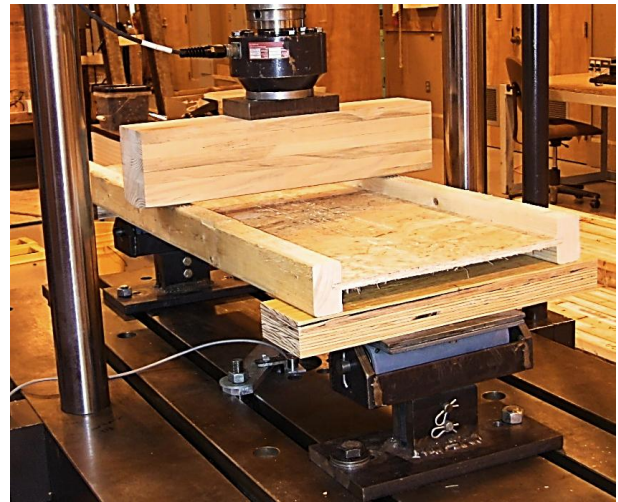
Figure 4-6: Lateral bending stiffness test configuration (inches).
