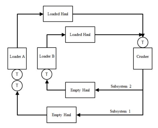
Figure 3.7: Queuing Schematic with Multiple Pits
