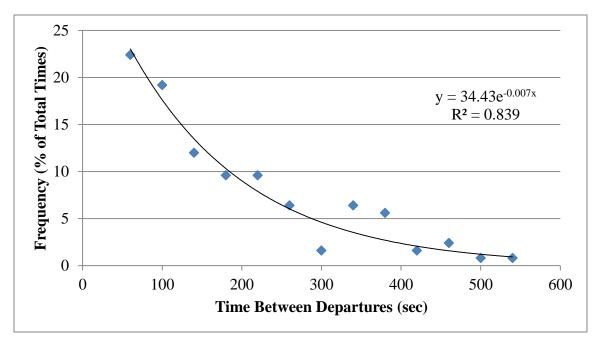
Figure 3.17: Service Distribution for a Single Loader
