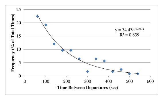
Figure A-5: Overall Service Distribution with 3 Loaders in Operation
