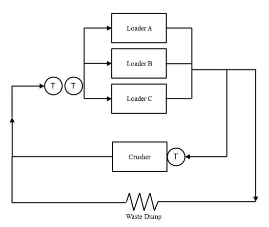
Figure 3.18: Queuing Schematic of Mine Haulage Route
