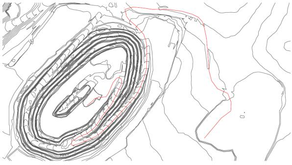
Figure 3.12: Haul Route from Pit to Waste Dump Location
