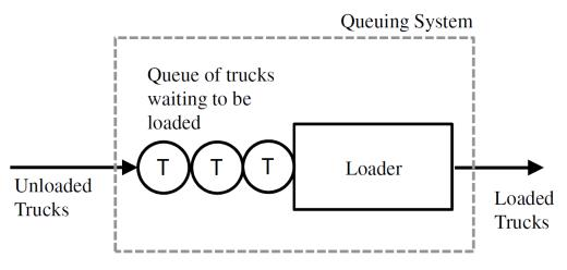
Figure 3.3: Truck and Loader Queuing System
