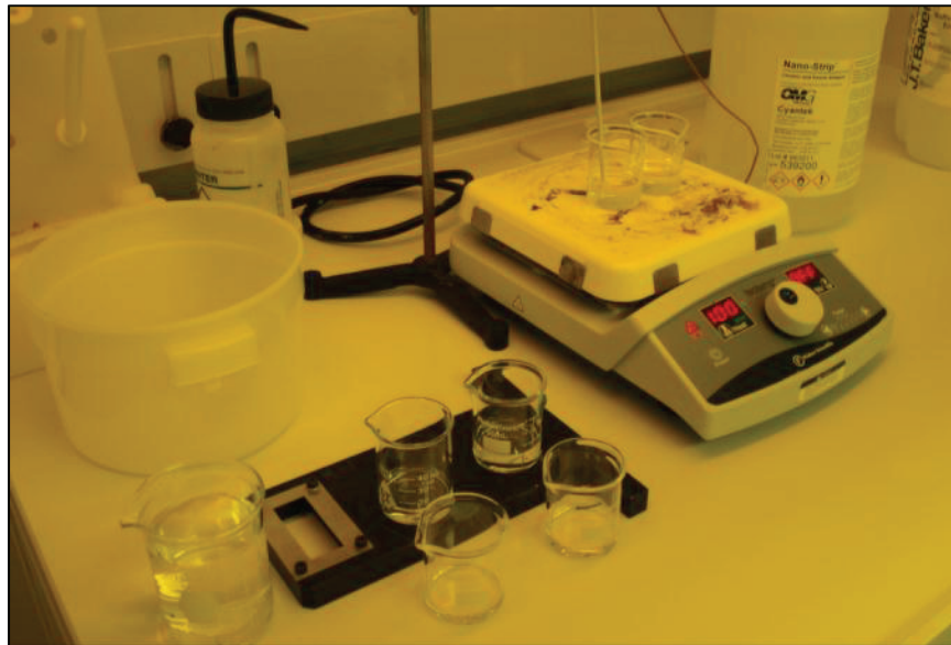
Figure 4-32: Fume hood set-up of Nano-Strip solution, hot nitric bath, and sulfuric acid wash in preparation for fiber cleaning in the Whittemore Hall clean room
