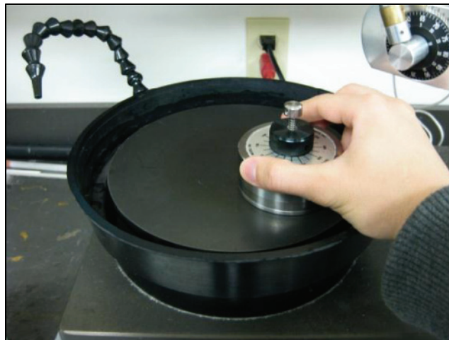
Figure 3-8: Hand polishing sapphire wafers was accomplished using a polishing platen to maintain wafer parallelism on a polishing wheel [18]
