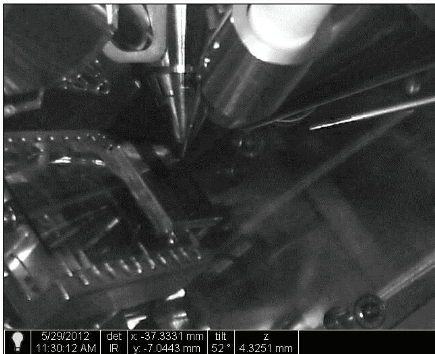
Figure 4-19: Helios NanoLab vacuum chamber internal camera image of stage tilted to 52 degrees
