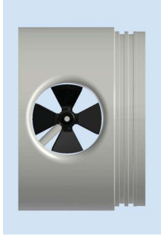
Figure 3. SPU Bow-Thruster Concept. This thruster design features a ducted propeller embedded in submarines hull. The location of the propeller eliminates any unwanted torques on the sub due to thrust or drag forces. The drawback is this type of thruster only provides thrust in the port and starboard directions.
