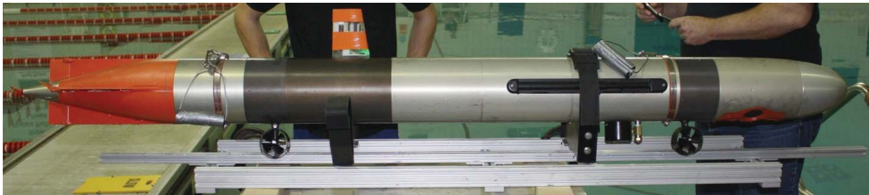
Figure 32. Virginia Tech 690 AUV with Integrated SPU Thrusters. The SPU tube sections can be seen aft of the submarine head and forward of the tail section. The lower housings and ducted propellers suspend below the body of the sub.
