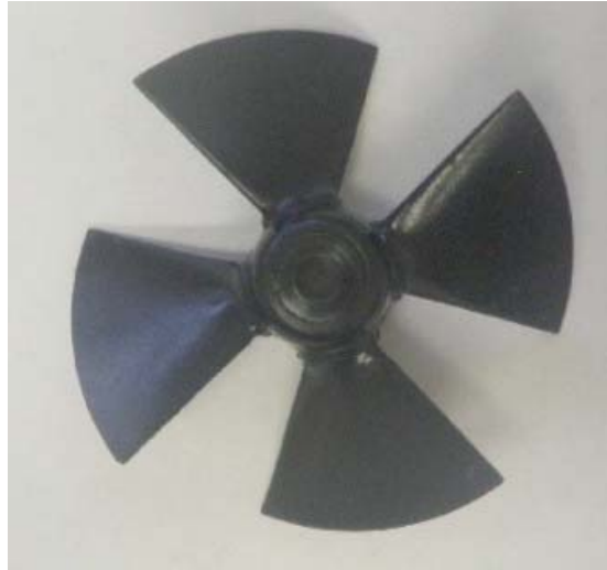
Figure 9. Graupner Hub Driven Propeller. This prop was used as a basis for the design of the rim driven prop.
