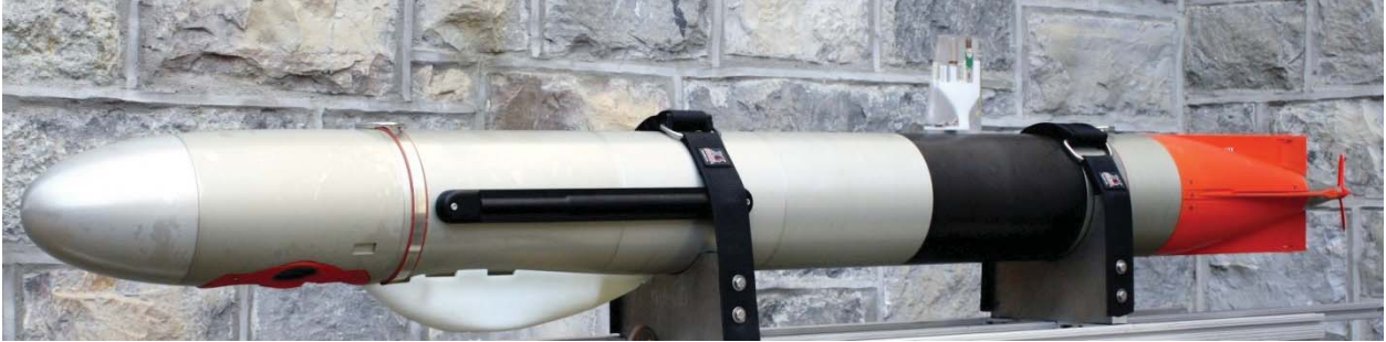
Figure 1. Virginia Tech 690 AUV. The Virginia Tech 690 is a miniature submarine AUV designed for the purpose of conducting general purpose ocean surveying missions.
