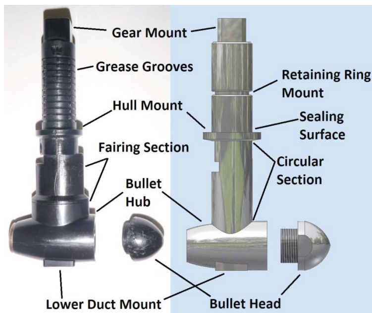
Figure 22. Graupner and SPU Lower Housings. (left) The Graupner lower housing was made of ABS plastic and had many features that prevented it from being implemented in the SPU.
