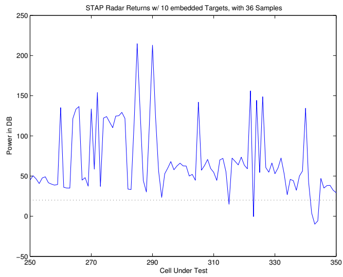
Figure 5.10: N = 33 , 10 outliers, K = 36 . In this case, the noise floor is too high and false targets are detected.
