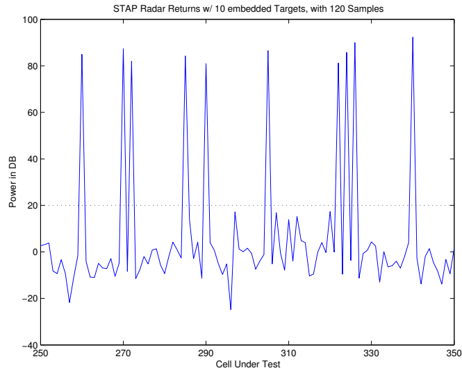
Figure 5.12: N = 33 , 10 outliers, K = 120 . The noise condition was suppressed and targets were revealed. However, there is not much further suppression beyond the theoretical optimal sample support.
