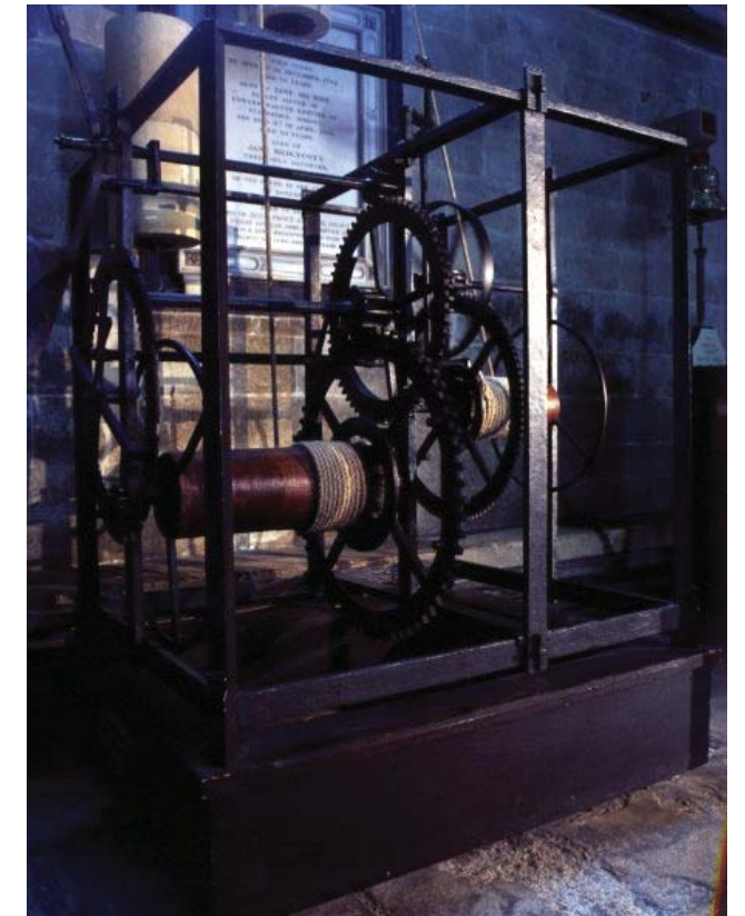
[26] Clock in Salisbury Cathedral. One of the earliest mechanical clocks.
