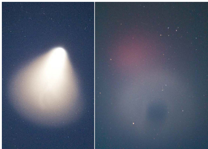
Figure 1.4: Images of the CARE I dust and molecular exhaust release showing (left) sunlight scattered from the aluminum oxide particulates and (right) dust ring produced by motor coning along with red-line emissions from excited atomic oxygen [After Bernhardt et al. , 2011].
