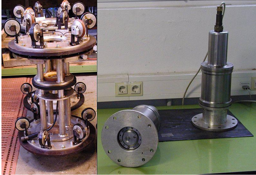
Figure 6 - Ultrasonic measuring heads are utilized on this crack detection pig [Public Domain]
