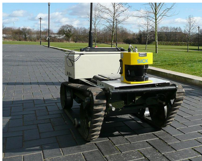
Figure 13 - Shown is a mobile robot equipped with a SICK single plane laser scanner. [Public Domain]
