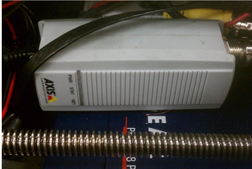
Figure 47 - Displayed is the AXIS video encoder used to encode the drive camera video feeds.
