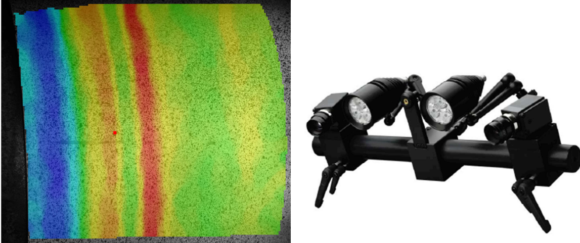
Figure 3.4: The random paint pattern applied to the box with axial strain output overlaid (left). A GOM ARAMIS DIC camera system (right). Used with permission of Trillion Quality Systems [19].
