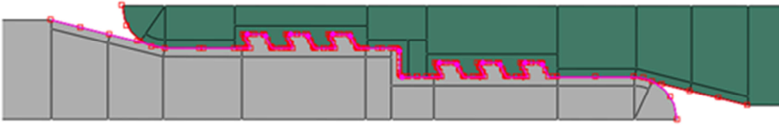
Figure 4.14: Master box contact surface shown in red. Slave pin contact surface shown in pink.
