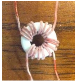
Figure 3.8 Transformer made of low loss toroid core
