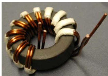
Figure 2.5 Toroid sample with bifilar winding
