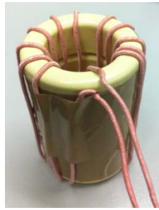
Figure 2.19 Choke inductor with stacked cores
