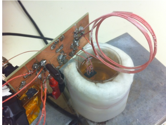
Figure 3.34 The inductor loss measurement setup
