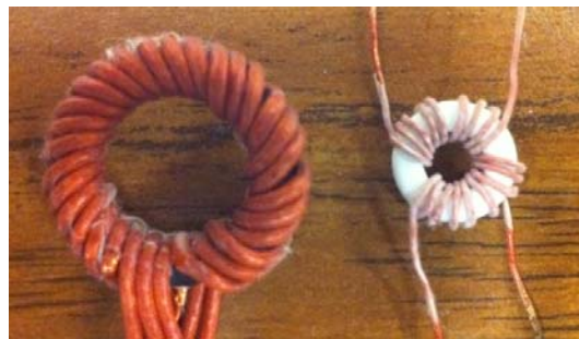
(a) Core under test (LTCC, left) and reference core (NiZn, right)
