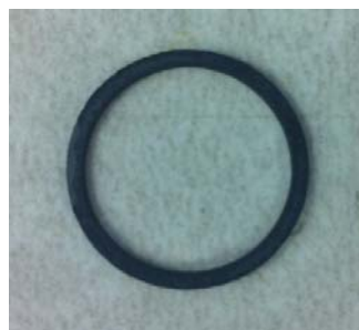
Figure 5.6 Sintered core sample
