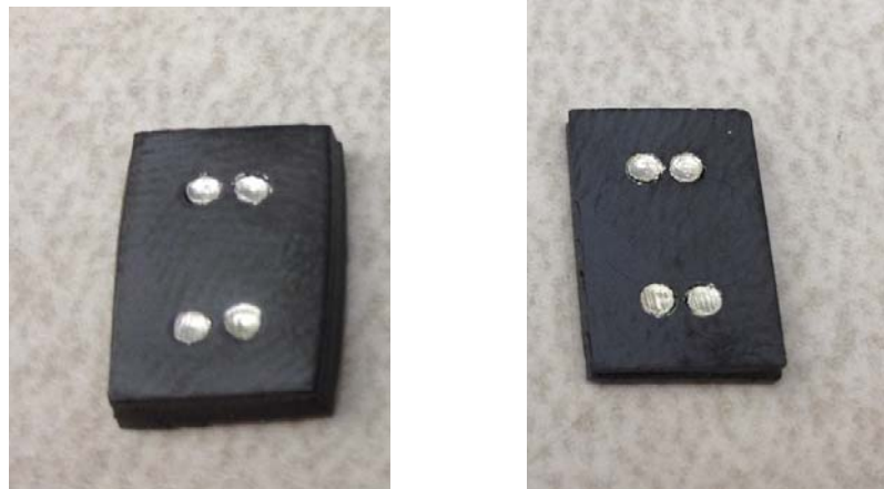
Figure 5.28 Planar inductors made of ESL LTCC 40010 (left) and L-LTCC 80 (right) (ESL 40010, h=2.3\text{mm} ; L-LTCC 80, h=1.65\text{mm} )
