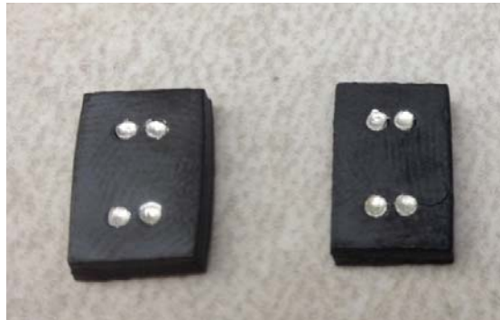
Figure 5.25 Two-turn planar inductors made of ESL LTCC 40010 (left) and L-LTCC 80 (right) with the same thickness ( h=2.3\text{mm} )
