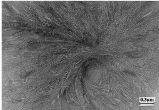
Figure 5.11 – Bright field TEM image of it-PS isothermally crystallized at 160°C for 6 hours and subsequently held at T_b for 1 minute 70
