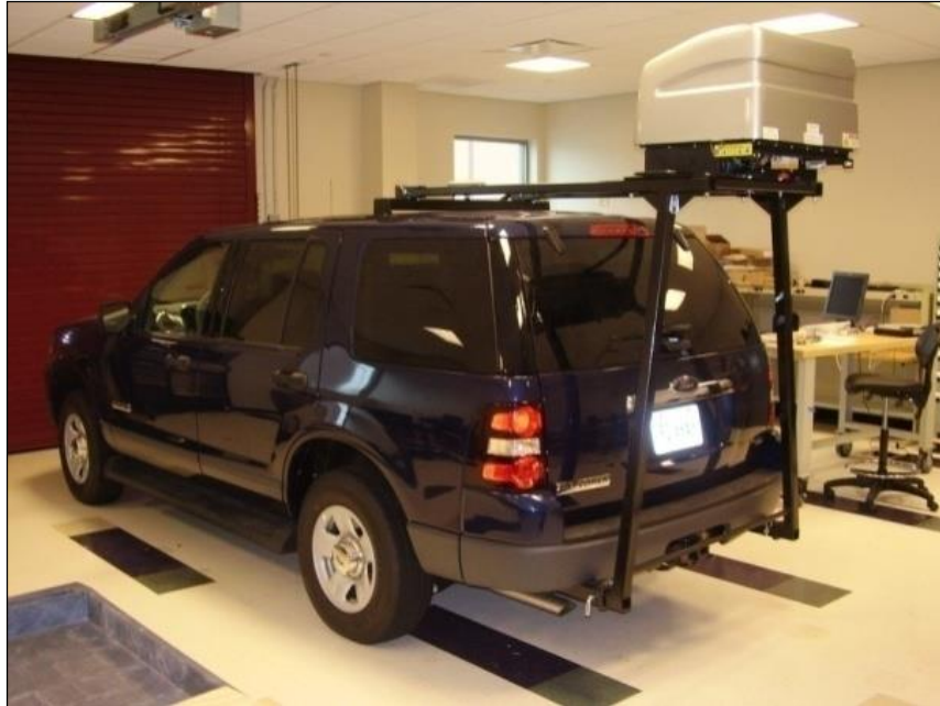
Figure 2-2. Vehicle Terrain Measurement System (VTMS).
