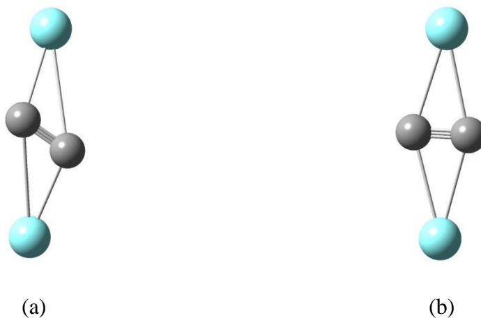
Figure 31: Two views of the modeled cluster geometry for Y_2C_2@C_{92} . The left view (a) is the optimized structure while the right view (b) is the transition state structure between two equivalent optimized structures.
