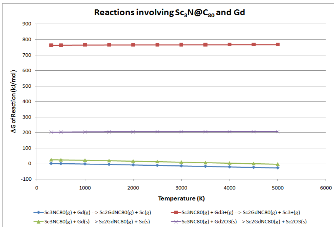
Figure 48: Plot of computed \Delta G of reaction versus temperature for reactions involving \text{Sc}_3\text{N}@C_{80} and gadolinium in several forms. Crystal entropy effects are not included for the oxide case.
