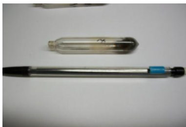
Figure 44: Sealed quartz tube containing \text{Sc}_3\text{N}@C_{80} and Al powder for attempted metathesis reaction.
