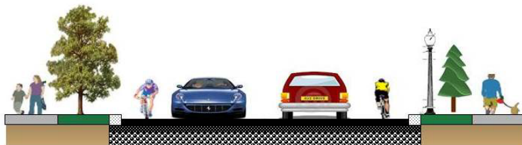
Figure 2: Standard cross section of an urban roadway
