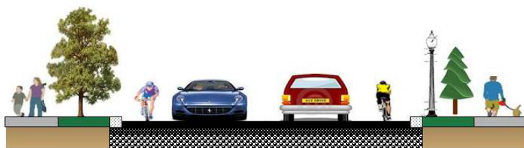
Figure 2: Standard cross section of an urban roadway
