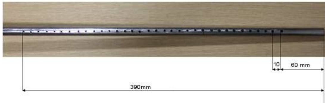
Figure 32. Stainless steel tube for gas sampling inside the enclosure.
