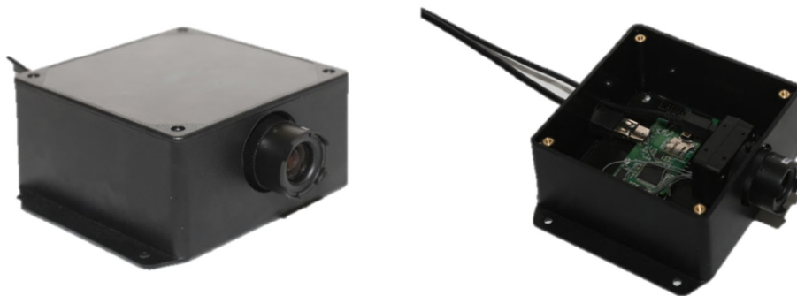
Figure 9: Sensor rig consisting of IMU and camera
