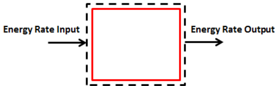
Figure 1.2 A system with a boundary, an input and an output.
