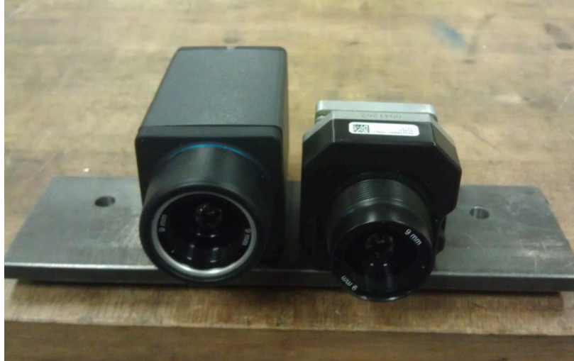
Figure 3. LWIR cameras used, FLIR A35 (left), FLIR Tau 2-320 (right)
