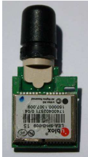
Figure 4.6: GS407 GPS Receiver unit used for gathering position information of UAV.
