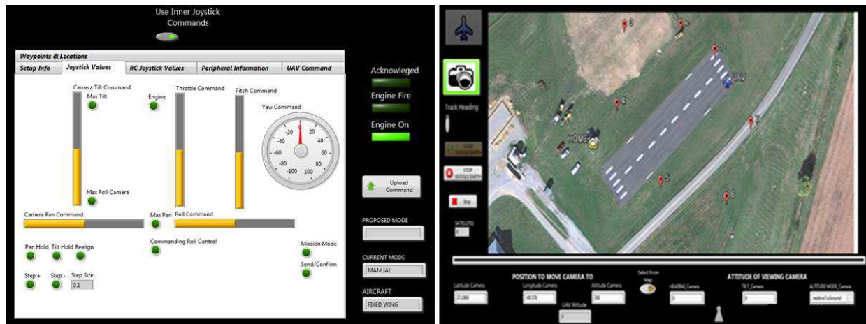
Figure 3.23: This image highlights two screens from the developed TCP Groundstation. The left image shows the joystick interface screen that relays flight commands to the UAV. The right image shows a sample flight path and UAV position in an embedded Google Earth window within LabVIEW.
