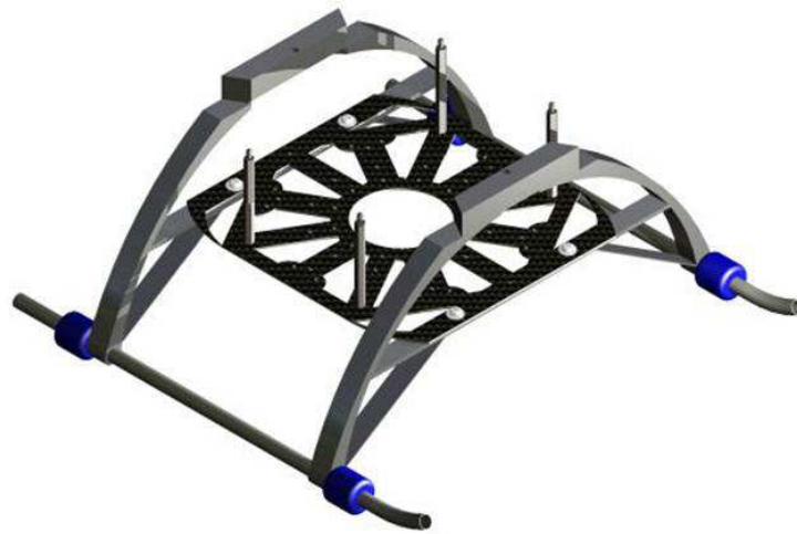
Figure 3.9: CAD rendering of the undercarriage and landing gear assembly of the HexaCopter platform.
