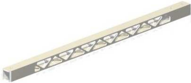
Figure 3.6: This figure shows a CAD rendering for each support arm of the HexaCopter.
