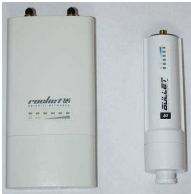
Figure 3.20: This figure shows the 5.8GHz Ubiquiti Network Radios used for this work. Left: Ubiquiti Rocket used for the ground side communications. Right: Ubiquiti Bullet used for the airside communications.
