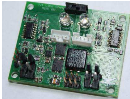
Figure 3.16: V1.0 of 5VDC buck regulator designed for system peripherals on the HexaCopter platform.
