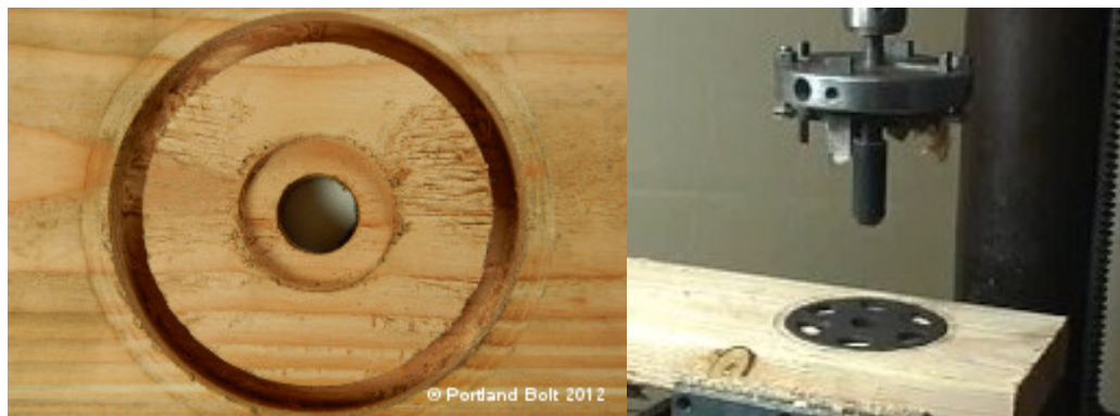
Figure 3.4: Grooves created by the dapping tool to accept the shear plate (left) and dapping tool above the shear plate which has been placed into the grooves cut by the tool (Portland Bolt & Manufacturing Company, 2012a)
