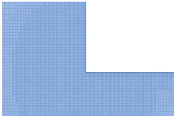
Figure 2. Corner and boundary layer mesh refinement
