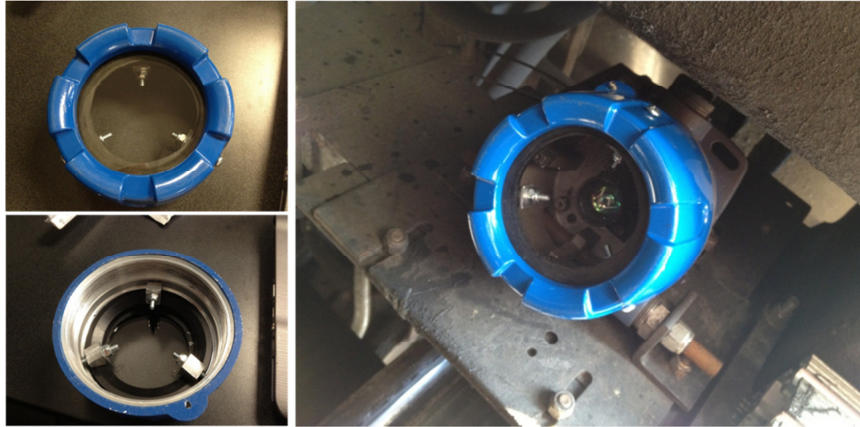
Figure 16: Explosion-proof protective housing securing the LIDAR lenses onboard the track geometry car
