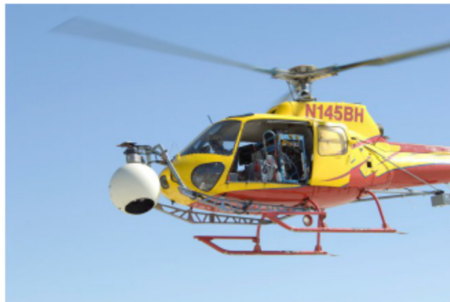
Figure 6: The LIDAR mounting for helicopter speed testing [17]
