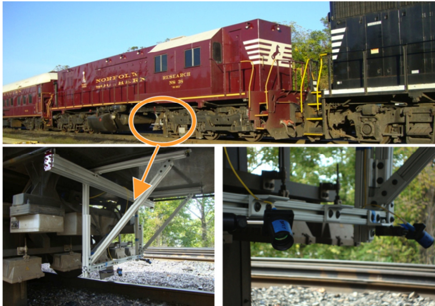
Figure 11: The LIDAR mounting setup on the track geometry car
