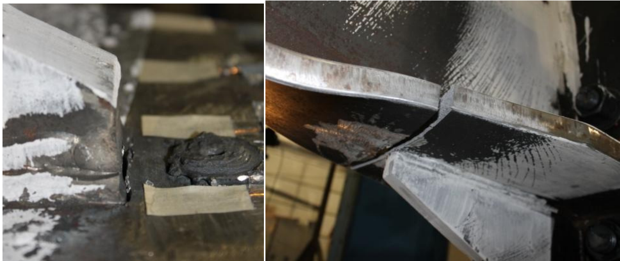
Figure 45: Stiffener Weld Metal Tear (left) and Bottom Flange Fracture Following Tear (right) from Test 8
