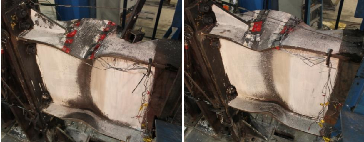
Figure 51: Deformations at 4.7% Story Drift for Test 10 (left) and Test 11 (right)
