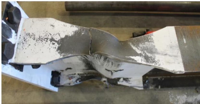
Figure 33: Brittle Bottom Flange Fracture from Test 5
