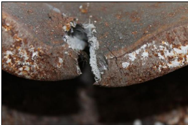
Figure 28: Ductile Flange Tear from Test 1
