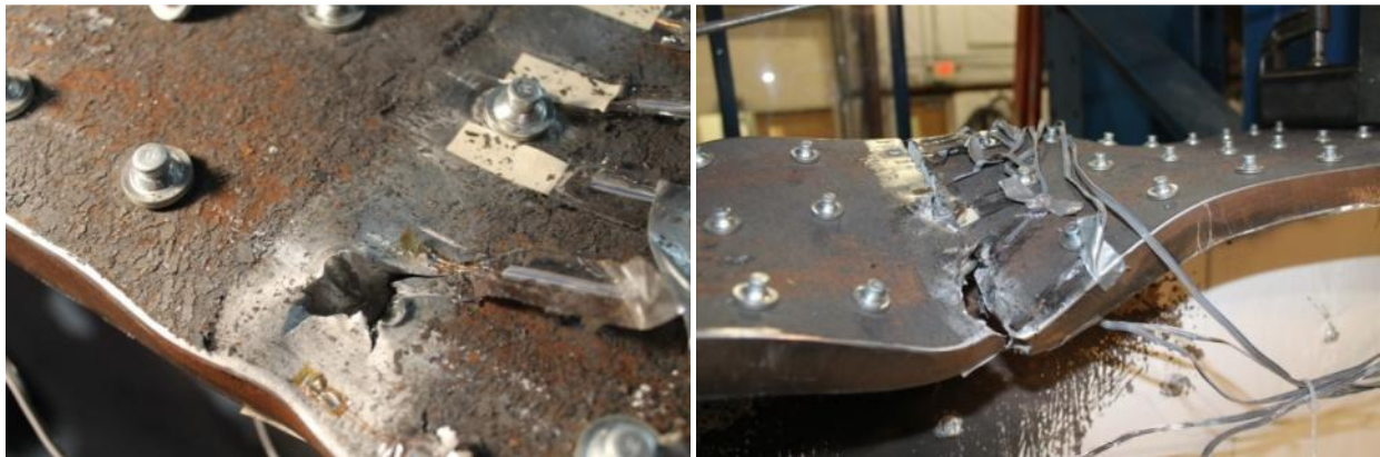
Figure 48: PAF hole during last 4% cycle (left) and full fracture during first 4.7% cycle (right) from Test 9
