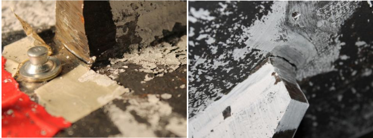
Figure 53: Tearing at Top Flange (left) and Bottom Flange (right) Endplate Stiffener Toe Welds from Test 11
