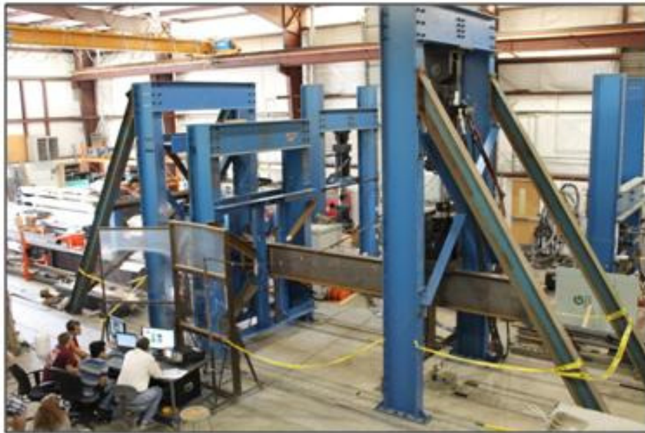
Figure 11: Full-Scale Test Frame
