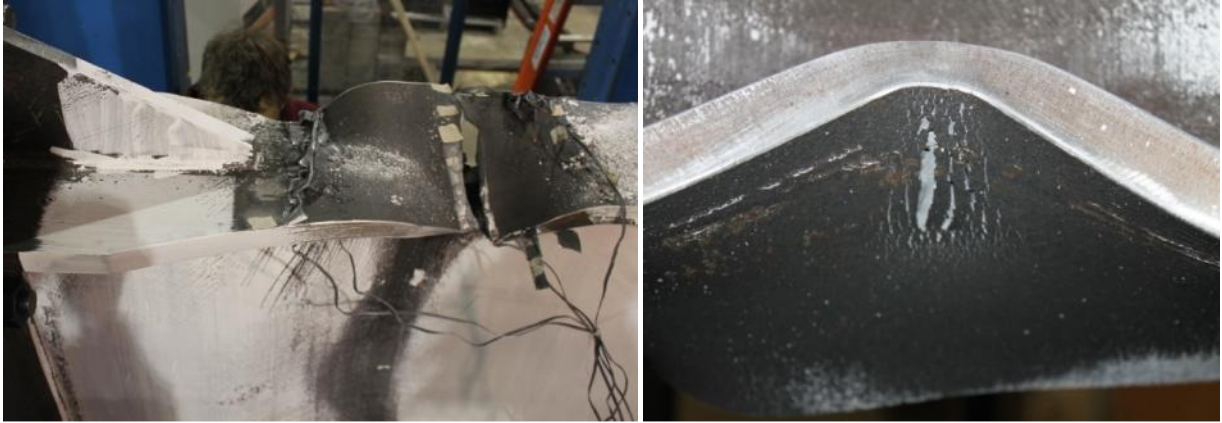
Figure 43: Brittle Fracture (left) and Tear Formation on the Underside of Bottom Flange Local Buckle (right) from Test 7
