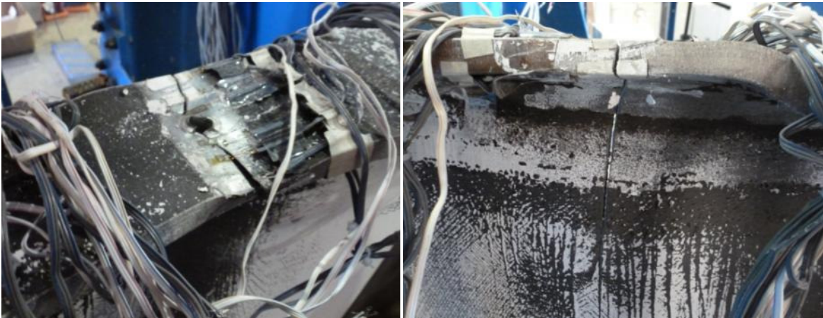
Figure 30: Brittle Flange/web Fracture from Test 2
