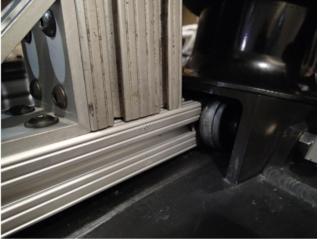
Figure 4-10: Wheels of suspension lifting tool wedged under airspring platform
