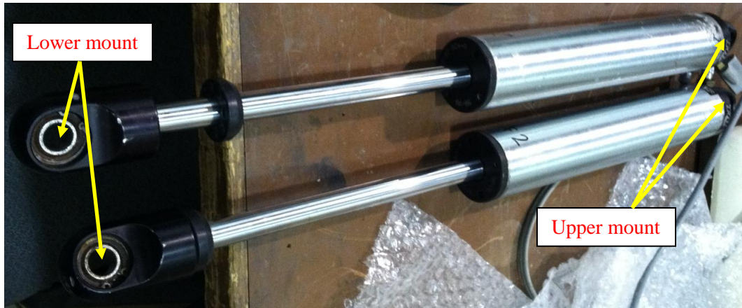
Figure 3-2: 33ft WAM-V stock dampers
