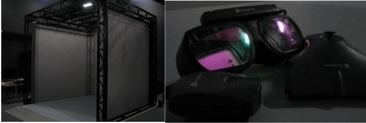
Figure 3.3: The VT Visionarium VisCube (L), and stereo glasses with a mounted IS-900 wireless tracker (R).
