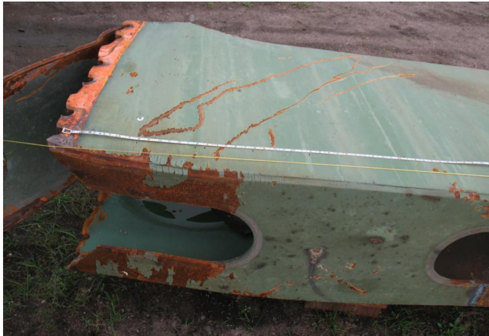
Figure 4.4-2: L9 end of the bottom chord segment L9-L10 recovered from the wreckage
