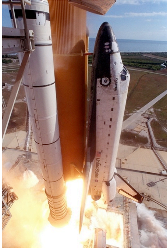
Figure 2-6. KSC Launch of Columbia STS 107. Reinforced carbon/carbon protects the wing leading edges on this vehicle. (CAIB photo by NASA, January 16, 2003 [17])
