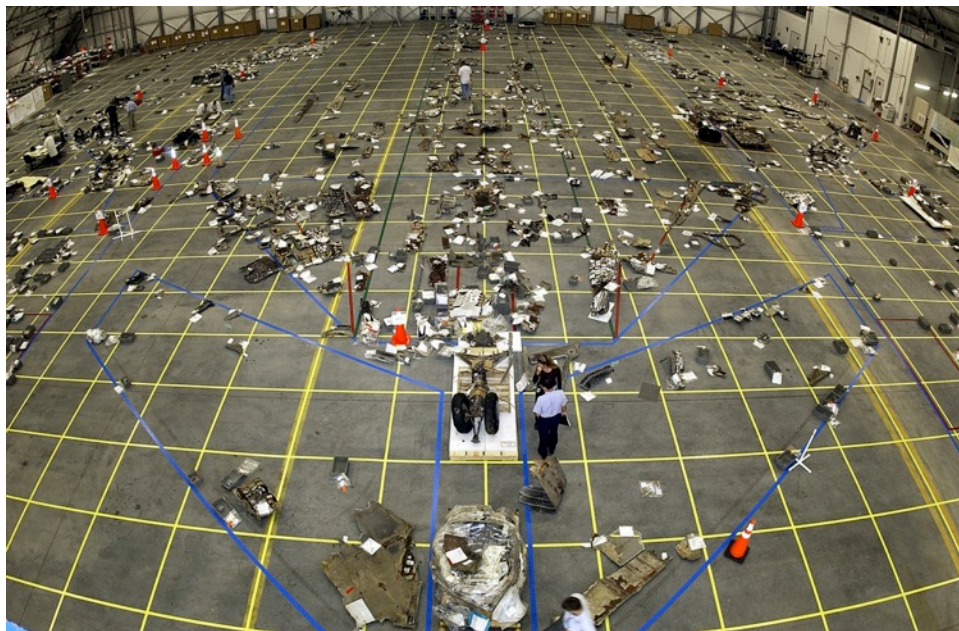
Figure 2-8. Recovered Columbia debris after break-up during re-entry. (CAIB photo by NASA, March 18, 2003 [19])
